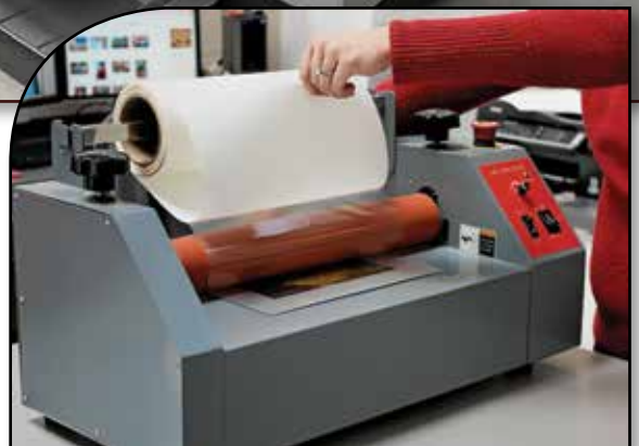
Lamination protects printed AlumaJet from moisture, abrasion and UV.
