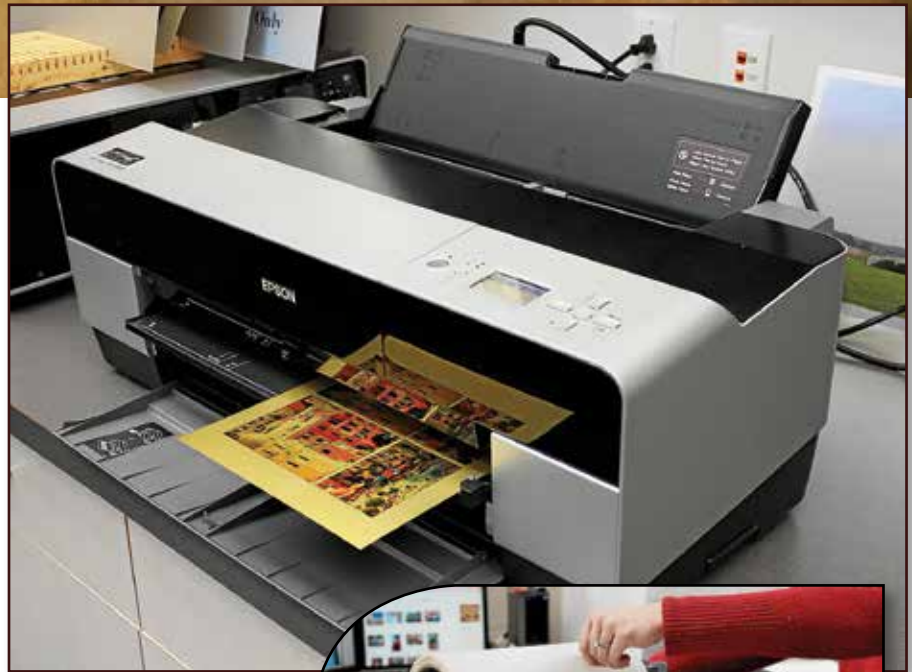
Epson 17-inch printer with straight through media path can print 0.025 AlumaJet sheets.
